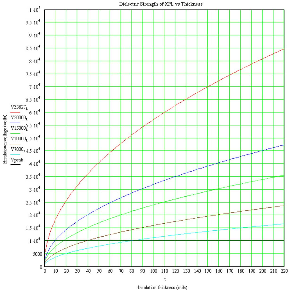
The top red trace (V35827) represents the dielectric strength (V/mm) of new XPL cable. Note that the breakdown voltage for 220 mil insulation is 84,691 volts. Penetrating this insulation with the URD Probe™ needle by even as much as 20 mils only reduces the breakdown voltage from 84,691 volts to 80,749 volts.
