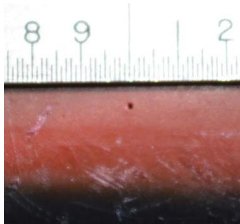
This small 10 mil hole is certainly very benign compared to the fact that unjacketed cable (illustrated below) has no jacket at all over its entire length. Unjacketed cable has been used for decades and hundreds of thousands of miles of this cable are still in service.
