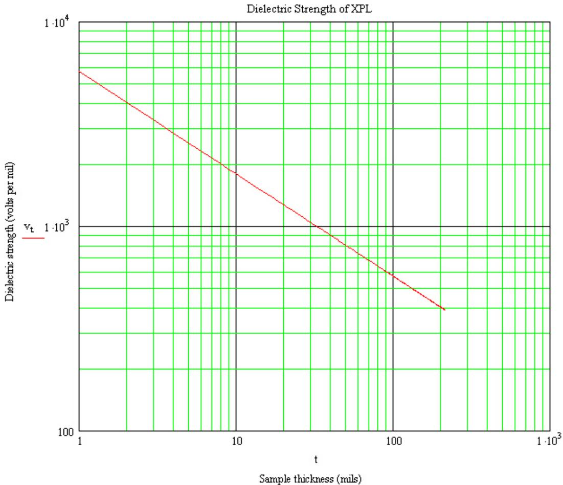
This graph illustrates that dielectric strength is not linear with thickness. The breakdown voltage of a 1 mil thickness is 5,711 volts. For a 2 mil thickness, it is 4,038 volts per mil times 2 mils or 8,076 volts. For a 10 mil thickness it is 1,806 volts per mil times 10 mils or 18,060 volts.
